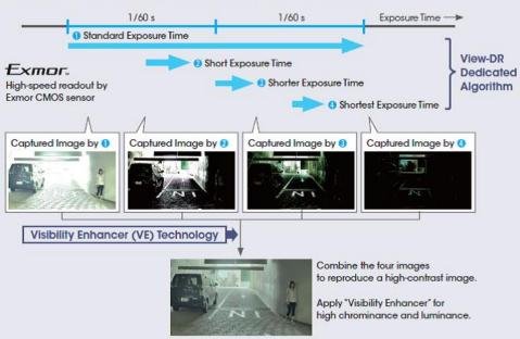
The full-capture wide dynamic range technology shall use an electronic shutter to capture multiple images and reproduce each frame.
